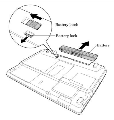
Figure 4-1 Removing the Battery pack
